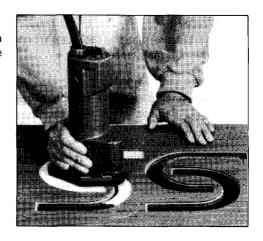
To install the templet guide, loosen the screws on the tool base, insert the templet guide and then tighten the screws.
